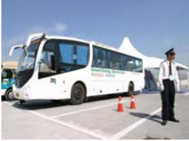
Electric bus in China - powered by Li-batteries (ThunderSky)
