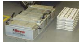
The size of lead acid batteries compared to ThunderSky Lithium batteries
