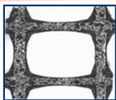
Each cell (400 per sq. in.), contains a washcoat and catalyst coating
