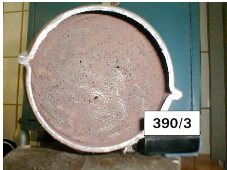
Figure 2. Red manganese deposits in China on a catalyst with cell density of 390/3 (catalyst channels/cells), after 20,000 miles of use. Higher cell densities (providing greater active surface area for more efficient conversion of pollutants) of 900/2 will be required to meet advanced emissions standards and appear to be even more prone to plugging. Source: Schindler 2004.
