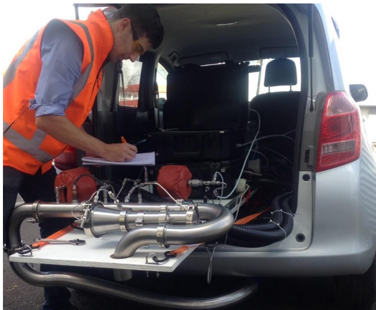
Figure 1. The PEMS equipment installed on one of the test vehicles.
